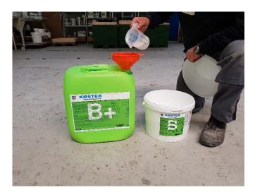
The mixed components can be processed for 2 hours.
